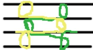
Along the spine (one needle). The needle enters each hole, creates a tie to the previous section and moves *along* to the next hole within the same signature.
